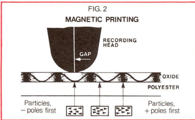
As frequencies of the electronic signal go higher into the treble region, the distance between the group of positive poles and negative poles becomes closer. Loudness depends on how deeply into the magnetic coating the arrangement penetrates and how many magnets it affects: the deeper it goes and the more magnets arranged, the louder the signal (FIG.3).
