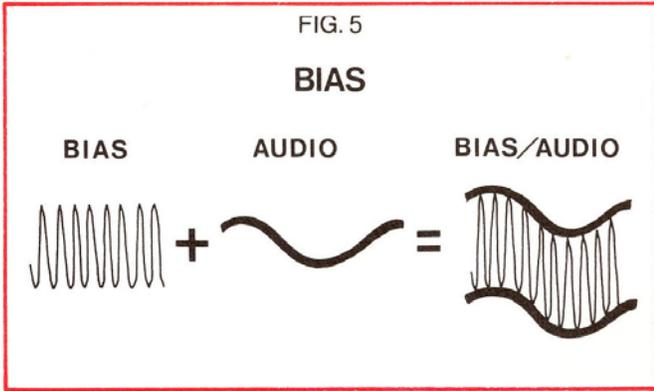
prints. The more coercive a tape, the harder it is to magnetize and the more bias it needs to get the particles to react without distortion. (Increasing bias does not raise its frequency — only its amplitude or strength or ‘loudness’ if it could be heard; the frequency stays the same.)
