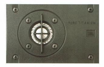
Being that thin, however, made the dome subject to deformation. And so JBL solved that problem by creating a patented, intricate network of ribs modeled directly into the dome. This ribbing increases the structural rigidity without increasing the thickness. And so, a dome 25 microns thick can be as strong as one that is 250 microns thick.
